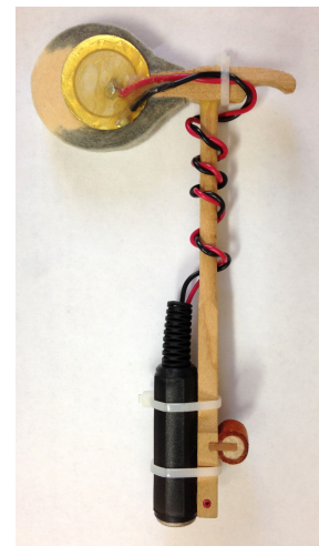
Figure 4: Piano action hammer with piezo element
