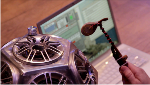
Figure 5: Hammer input device with hemisphere speaker
